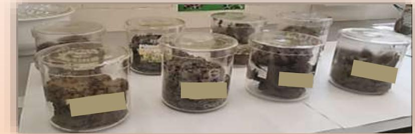
The soil samples were treated at the real treatment ratio used for tunnelling; Soil samples were collected and analysed at 3 different times (0, 14, 28 days)
